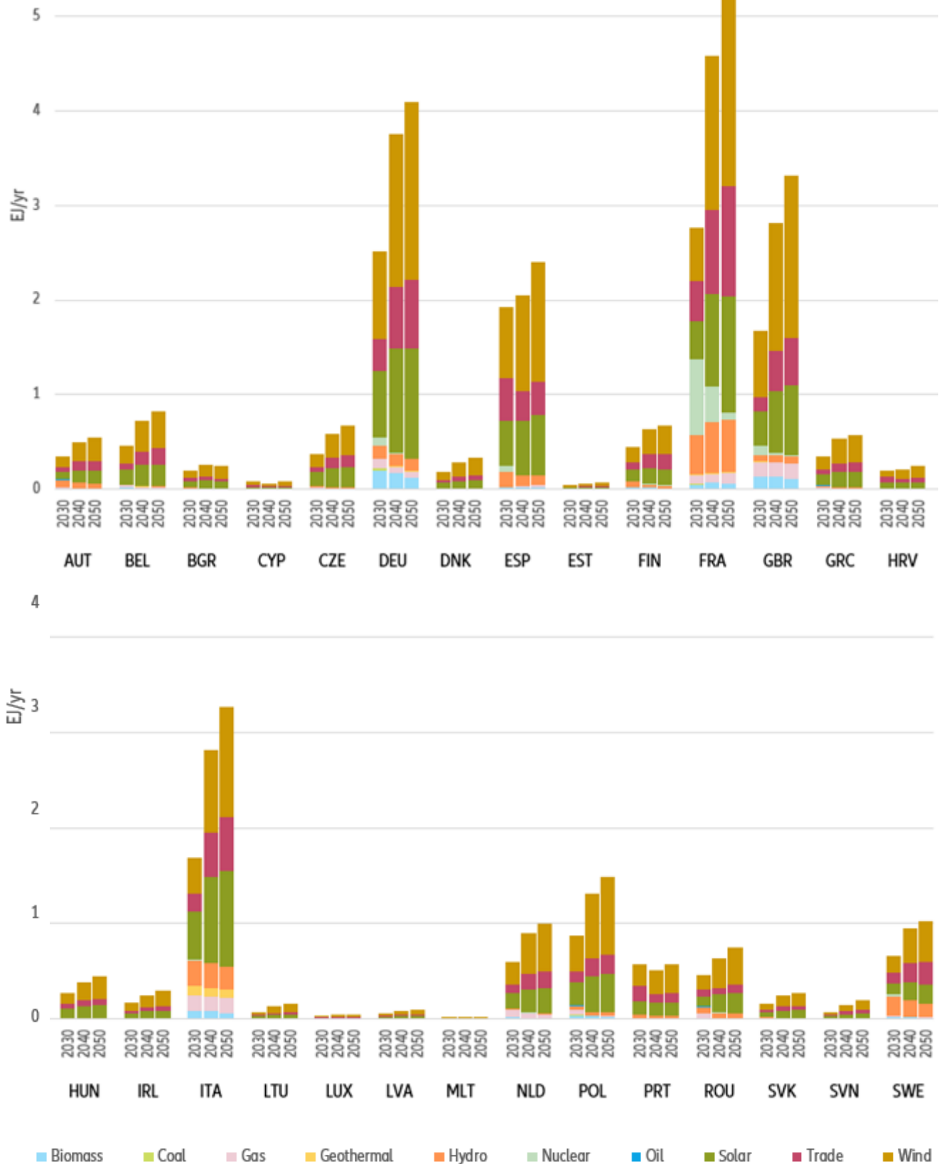
Figure 14: Evolution of electricity generation by technology in the EU-27 and the UK for reaching the 1.5°C goal
